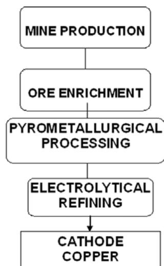
Figure 5. Basic technological scheme of copper pyrometallurgical production
